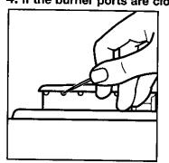
with a straight pin. Do not enlarge or distort the port. Do not use a wooden toothpick. If the burner needs to be adjusted, call a qualified technician for service.
